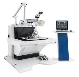
The laser and movement system are easily ope-rated from a side console with an intuitive touch screen. You can choose to weld manually with the quick-reacting joystick, semiautomatically or automatically with WINLaserNC software.
