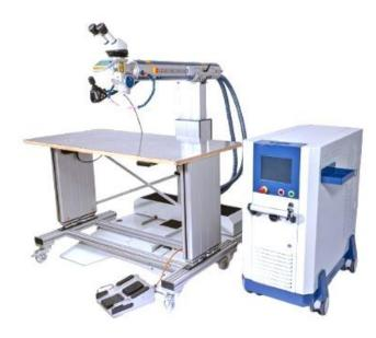
The special feature of the AL-IN is that it is not the workpiece that is moved, but the resonator. The axes are moved via the joystick, the touch display, or the AL-DRIVE\* control unit.
