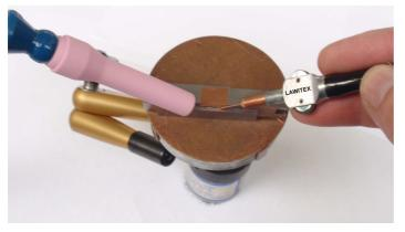
Fast and precise positioning of workpieces with the flexarm.
